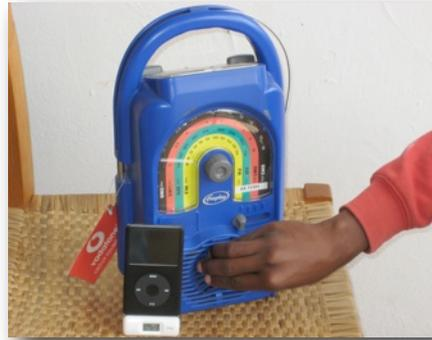
Equipping schools with a low-cost, portable transmitting device that allows “broadcasting” from the MP3 player to the radio. This eliminates the need for external speakers and allows teachers to continue using radios already distributed by the project to community schools throughout the country.
